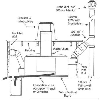
Locations where the monthly Relative Humidity exceeds 80% at any time, a vent drain and insulation of the outlet vent should be installed to ensure condensate does not re-enter the Rota-Loo.
