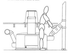
Enough space around the Rota-Loo to connect the Air Inlet, Vent pipe and to maintain the Rota-Loo once installed.
