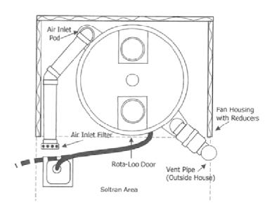
Allow also sufficient space to permit fitting insulation around the Rota-Loo. This is essential in cold climates.
